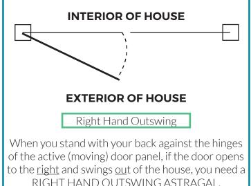
Astragals should be ordered based on the handing and swing of the active (moving) door panel.
