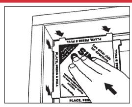
a. Peel back the weatherstrip from the header and jamb in the corner where you are working. Position the pad in an upper corner of the frame so that the tab-like protrusions meet the jamb & header.
