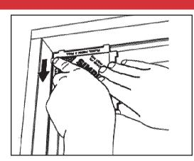
b. Once aligned - press pad firmly onto rabbet stop of the side jamb and head jamb to fully adhere the part to the jamb surface.
