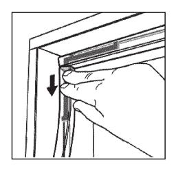
Insert the head jamb and side jamb weatherstrip as normal. Repeat process for other corner.
