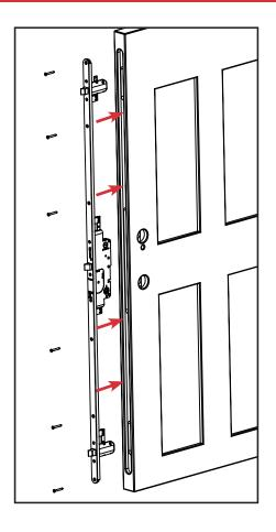
Place the new lock face out into the channel. Ensure the lock faceplate is flush with the panel. Screw the lock in using the screws provided.
