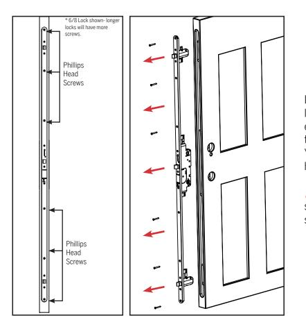
Loosen the screws that secure the lock on the panel and remove the existing lock. Clear out any debris that may be in the exposed channel. You do <u>not</u> need to remove the torxhead screws.
