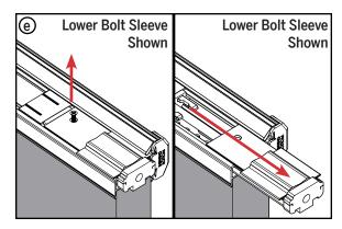
**e.** Remove the screw securing the lower bolt sleeve and slide the bolt sleeve out.
