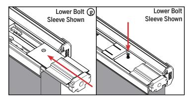
**g.** Return the bolt sleeve onto the lower bolt and reinstall the screw securing the bolt sleeve.
