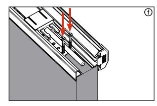
**f.** Install two #8 x 1" screws on either side of the bolt pin above the U-Shaped cutout in the astragal body.
