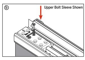
**b**. Remove the orange securing pin from the upper bolt sleeve and replace it with a #8 x 1-1/2" screw.
