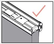
Ensure the upper and lower bolts are in the retracted position.
