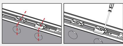
Secure the strike and deadbolt plates in their proper location by aligning them with the crossbore holes and tighten the screws into the retainers.
