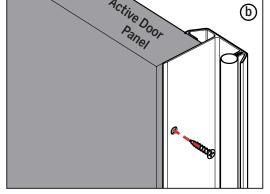
**b.** Insert the screws through the predrilled holes to secure the flange snug against the face of the active door.
