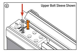
**a.** Keeping the orange securing pin in place on the upper bolt sleeve, install a #8 x 1-1/2" screw in the hole adjacent to the orange securing pin.
