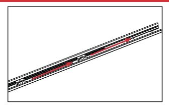
a. Slide the strike retainer out of the astragal. If you are replacing the deadbolt retainer, slide this out of the astragal body as well.
