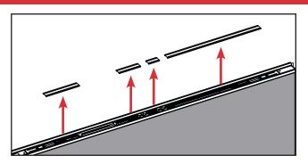
b. Remove the trim strip along the entire astragal body to expose the screws that secure the astragal on to the door panel. Note where the 4 pieces of the strip belong, as you will have to return them to the exact position.
