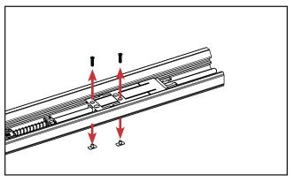
b. Screw the shoot bolt in place using the T-nuts and smaller screws in the smaller screw holes.
