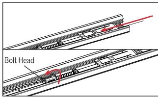
a. Slide the bolt assembly into the astragal body. Rotate the bolt head into the exact position from which the previous bolt was removed.
