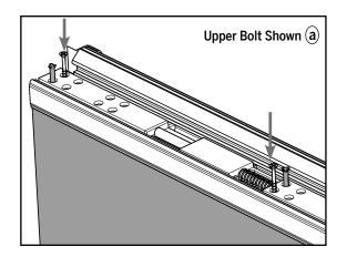
**a.** Keeping the orange securing pins in place on the upper bolt, secure two #8 x 1-5/8" screws in the holes adjacent to the pins.
