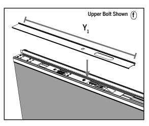
**f.** Keeping the cutout aligned, cut the trim strip to match  $Y_1$  and install in the upper part of the astragal.
