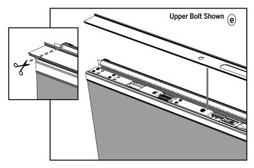
**e.** Align the D-shaped cutout on the trim strip with the push button on the upper bolt. If there is an overhang past the top of the upper bolt, cut the trim strip to fit flush with end of the astragal.
