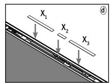
**d.** Cut the strike support trim strip into lengths matching  $X_1$ ,  $X_2$  and  $X_3$  and install each piece on the strike support.
