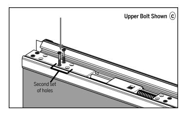
**c.** Insert two additional  $\#8 \times 1-5/8$ " screws into the second set of holes on the upper bolt sleeve where the holes align with the holes in the body.
