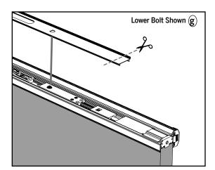
**g.** Align the D-shaped cutout on the trim strip with the push button on the lower bolt. If there is an overhang on to the lower bolt sleeve, cut excess trim strip.
