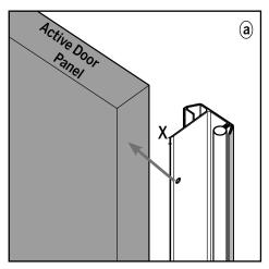
**a.** Position the security flange on the active door panel with the wide flange facing the outside of the house. Peel the tape backing and secure against the active panel.
