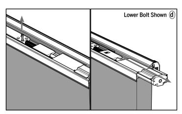
**d.** On the lower bolt, note the location of the orange securing pin and remove the pin. Slide the lower bolt out of the astragal.
