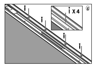
**g.** Locate additional screw holes in the astragal body and insert four #8 x 1" screws into these holes to secure the astragal to the door panel.
