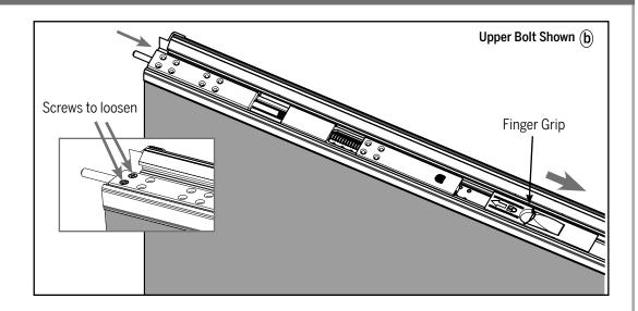
**b.** Retract the bolt by pulling the finger grip back. If retracting the bolt is tight on the upper bolt, loosen the screws on the upper bolt sleeve.
