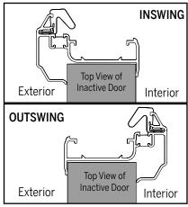
a. Align the astragal body flush with the end of the inactive door panel, with the wide side of the astragal correctly oriented based on swing of the door.For Inswing doors, the wide side of the astragal goes on outside of the door.For Outswing doors, the wide side of the astragal goes on inside of the door.
