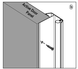
**b.** Insert the screws through the predrilled holes to secure the flange snug against the face of the active door panel.
