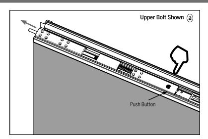
**a.** Press the push button on the upper and lower bolts to ensure the bolt pin is properly engaged.
