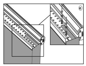
**e.** Add two #8 x 3" screws beside the U-shaped notch in the astragal body - one in the second hole from the bottom, and the other in the hole directly above the notch.
