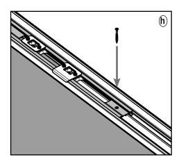
**h.** Return the strike support to its original location and screw back into place.
