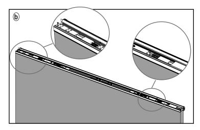
**b.** Press the astragal down along the length of the panel. Three orange securing pins will pop up - two on the upper bolt and one on the lower bolt. **Do not remove pins at this time.**
