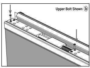
**b.** Replace the orange securing pins with #8 x 1-5/8" screws.
