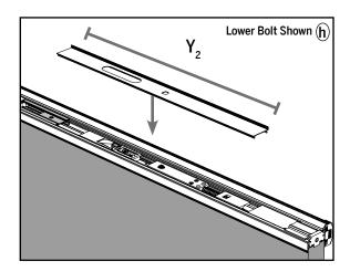
**h.** Keeping the cutout aligned, cut the trim strip to match  $\mathbf{Y}_2$  and install in the lower part of the astragal.
