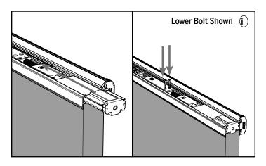
i. Slide the lower bolt back in place and install two #8 x 1-5/8" screws into the hole from which the orange securing pin was removed and the one adjacent to it.
