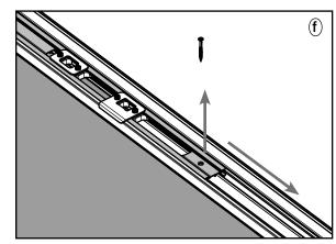
**f.** Remove the screw on the strike support and slide towards outside of the astragal body to gain access to screw holes in the astragal body.
