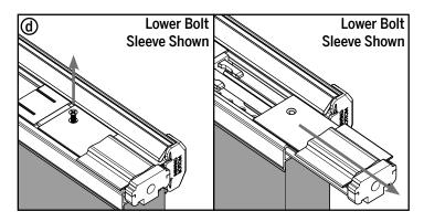
**d.** Remove the screw securing the lower bolt sleeve and slide the bolt sleeve out.
