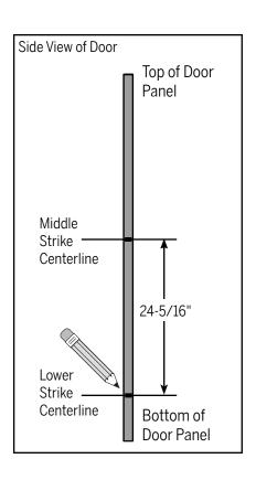
**c.** To determine the lower strike plate centerline, measure down 24-5/16" from the middle strike centerline toward the bottom of the door and mark.
