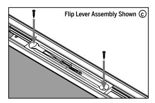
**c**. Install two #8 x 1" screws to secure the flip lever assembly into the door panel.
