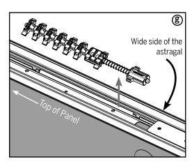
**g.** Remove the spine assembly and set aside to reveal screw holes in the body of the astragal. Remove by lifting from the wide side of the astragal first.
