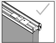
Ensure the upper and lower bolts are in the retracted position.
