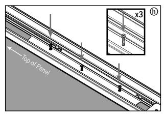
**h.** Install three #8 x 1" screws into the astragal body to secure the astragal to the door panel.
