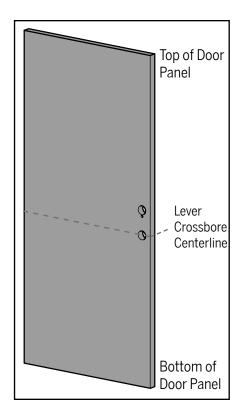
**a.** Determine the inactive door panel's lever crossbore centerline and mark.
