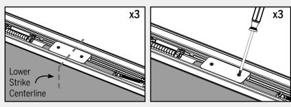
Adjust the location of the strike plates based on the three strike centerlines marked in Part A ( Page 2). Tighten the screws to secure them into place.
