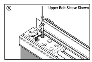
**b**. Remove the orange securing pin from the upper bolt sleeve and replace it with a #8 x 1-5/8" screw.
