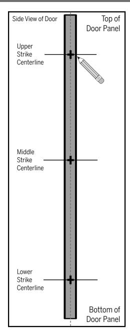
**e.** Determine the center point on the upper, middle and lower strike centerlines and mark the locations.
