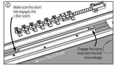
**i.** Return the spine assembly into the astragal, ensuring correct orientation as shown in image below.
