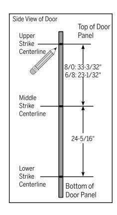
**d.** To determine the upper strike plate centerline, measure from the middle strike centerline up 23-1/32" for 6/8 doors or 33-3/32" for 8/0 doors and mark.
