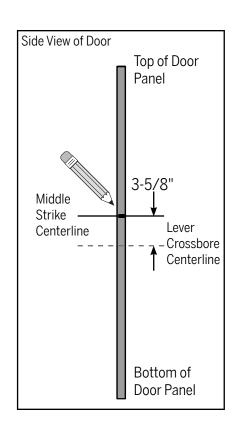
**b.** To determine the middle strike plate centerline, measure 3-5/8" up from the lever crossbore centerline towards the top of the panel and mark.
