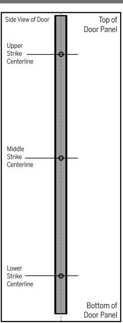
**f.** Using a 1" spade bit, drill a 1/2" deep hole at each center point. Clear debris from the holes.
