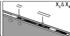
Middle Trim Strips: Install the X, trim strip to be flush between the bottom of the upper strike plate and the top of the middle strike plate. Install the  $\mathbf{X_3}$  trim strip to be flush between the bottom of the middle strike plate and the top of the flip lever assembly. Install the  $X_{\Delta}$  trim strip to be flush with the bottom of the flip lever assembly and the top of the lower strike plate.
