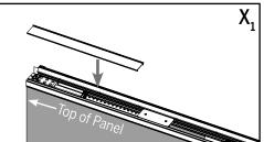
**Upper Trim Strip:** Install the  $X_1$  trim strip **Lower Trim Strip:** Install the  $X_5$  to be to be flush between the top of the astragal flush between the bottom of the lower and the upper strike plate.
