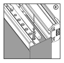
**e.** Install one #8 x 1" screw on the lower most hole next to the U-notch in the astragal body.
