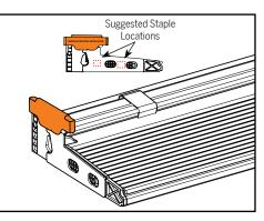
b. Staple the base onto the side in the locations shown. Repeat this on the other end of the sill with the other Z-End Base<sup>TM</sup>.
