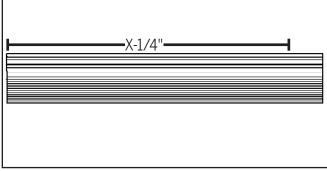
Measure and mark the new sill 1/4" less than the previous sill width. (X-1/4")
