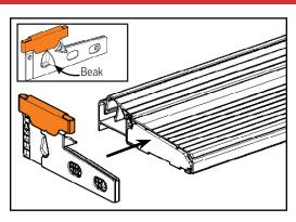
a. Place the Z-End Base<sup>™</sup> against the end of the uninstalled sill as shown in image. Align the stiffener's "beak" on top of the sill deck, adjacent to the cap.
