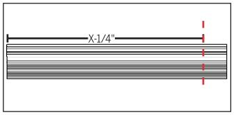
Using the mark you made (X-1/4"), cut the sill using a miter, chop or radial saw with a carbide tip blade.
