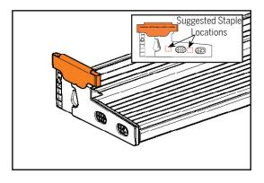
b. Staple the base onto the side in the locations shown. Repeat this on the other end of the sill with the other Z-End Base $^{\text{\tiny{M}}}$ .
