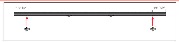
If necessary, reposition the spring-loaded center bases within the cap. To move the center bases, compress the spring in the base and then slide it. The center bases on the end of the caps should be 1" to 1-1/2" from the ends. The center bases should be evenly spaced.
