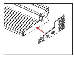
a. Place the sidelite stiffener against the end of the <u>uninstalled</u> sill as shown in image.
