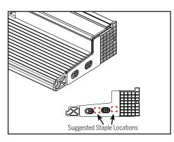
b. Staple the base onto the side in the locations shown. Repeat on the other side of the sill if a sidelite is present on that side as well.
