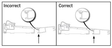
c. Double check that extender is in place correctly.
