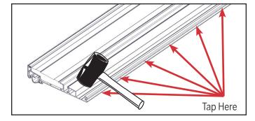
**b.** Using a rubber mallet tap the extender along the length of the sill to ensure the extender clips onto the sill.
